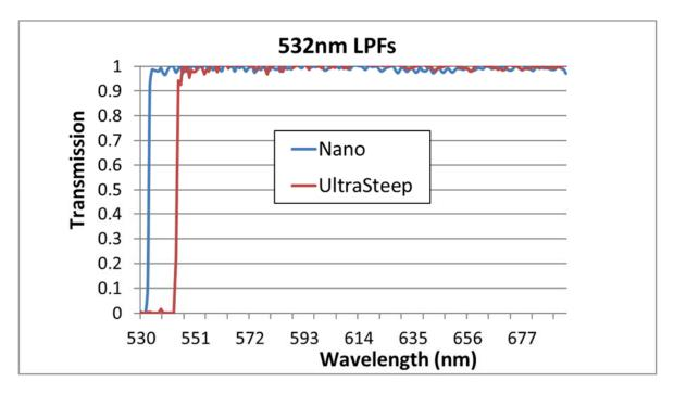
Iridian's wide angle long pass filters (WA LPF) are a preferred solution for customers' instruments and devices with wider AOI ranges of 0-2 degrees, CHA up to 5 degree, and provide extended passband wavelength range with transmission > 93-95%, and extended blocking wavelength range with OD6 blocking over the broad operating ranges of these devices.
