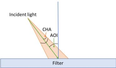
Field of view, or FOV, is the angular range over which a collimated or uncollimated beam is incident on the filter's first surface, measured relative to the surface normal at the surface that the beam is incident upon. While similar to CHA, a non-zero FOV may result from a convergent or divergent beam or a use condition in which collimated light may vary in its angle of incident over time.
