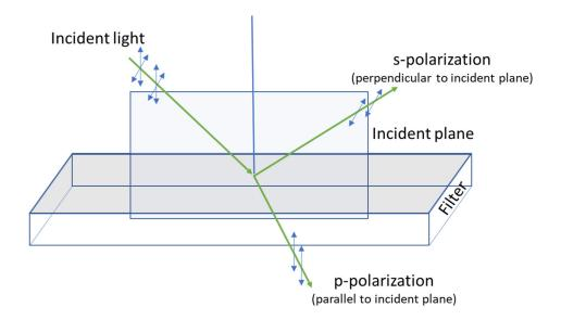
In many instances the incident light is unpolarized so the filter must be designed for use in random polarization (that is, all specifications need to be met for either s or p polarization state) but in cases where the incident light is polarized or where the filter functions as a polarizing beam splitter it is important to specify which polarization is relevant.
